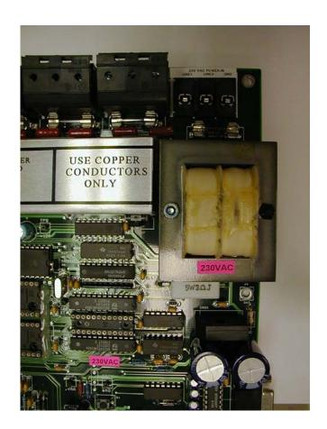
3. Referring to the picture below, turn the board over and connect a short bare solid wire between the two transformer pins on either side of the metal screw used to hold the transformer against the board. Then solder all eight pins of the transformer to the board. For added security you should encase the short bare solid wire with hot glue to prevent it from moving and touching the metal screw.
